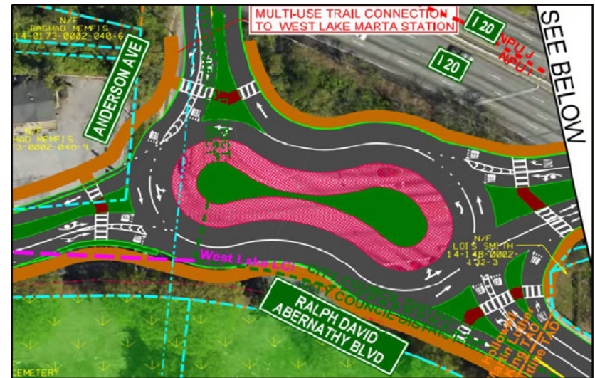
“Peanut-shaped” roundabout Arcadis developed for GDOT
