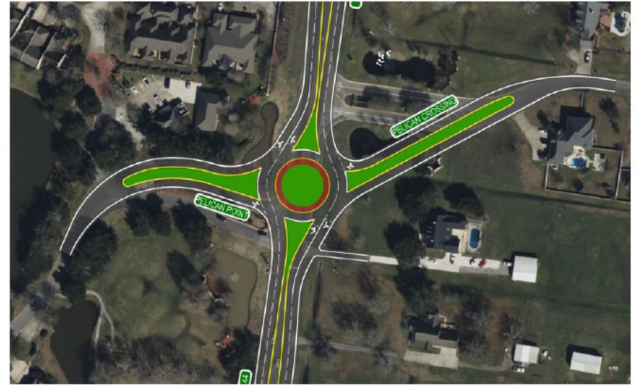
Potential design combining Pelican Point & Pelican Crossing Approaches into LA 44 Roundabout
